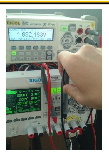
Ground the 2 lows together externally using shorted wires
