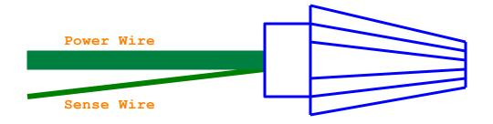
The Power Wire delivers the current, and the Sense Wire is fed back to the voltage from the Terminal.
