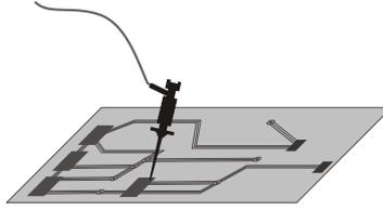
Figure 2-10 Attach the clip to testing point
