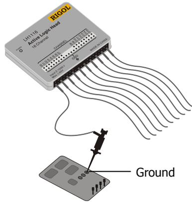
Figure 2-11 Connect to the ground
