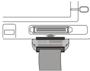
Figure 2-8 Connect the digital probes to oscilloscope
