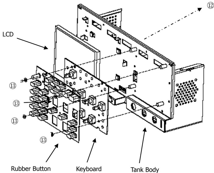
Figure 5-6 Disassemble and assemble LCD and the keyboard
