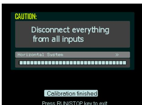
Figure 4-2 Finish Self-Calibration
