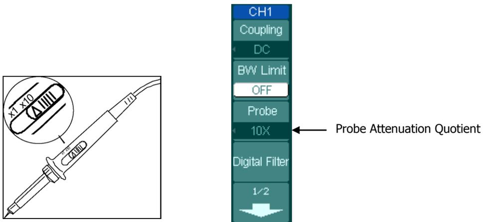
Figure 2-5 Set the probe attenuation quotient and switch
