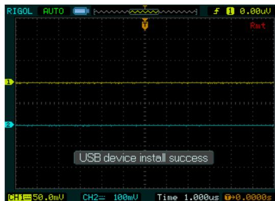
Figure 3-2 Successful prompt of USB interface connection
