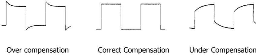
Figure 2-7 Waveform compensation
