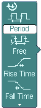
Figure 2- 127 Table 2- 82 The Time Measurements menu (Page 2/3)
