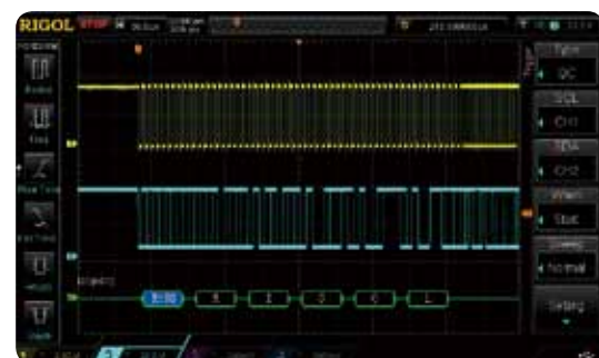
Optional Serial Bus Triggering and Decoding functions(RS232,I2C,SPI)
